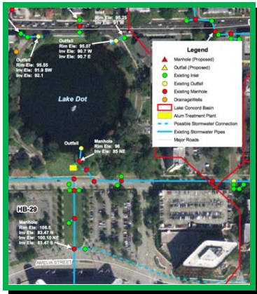
Outfalls, storm sewers, man holes, and alum treatment plant locations near Lake Dot.
