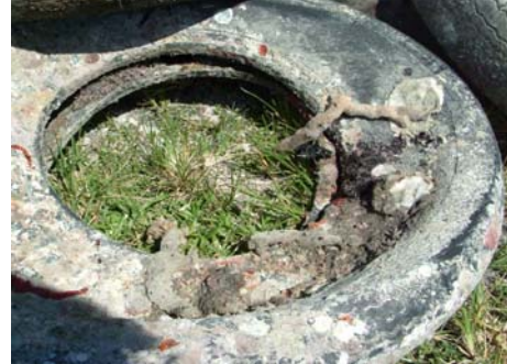
Figure 10. Higher organic contamination sample tires after 20 hours of drying
