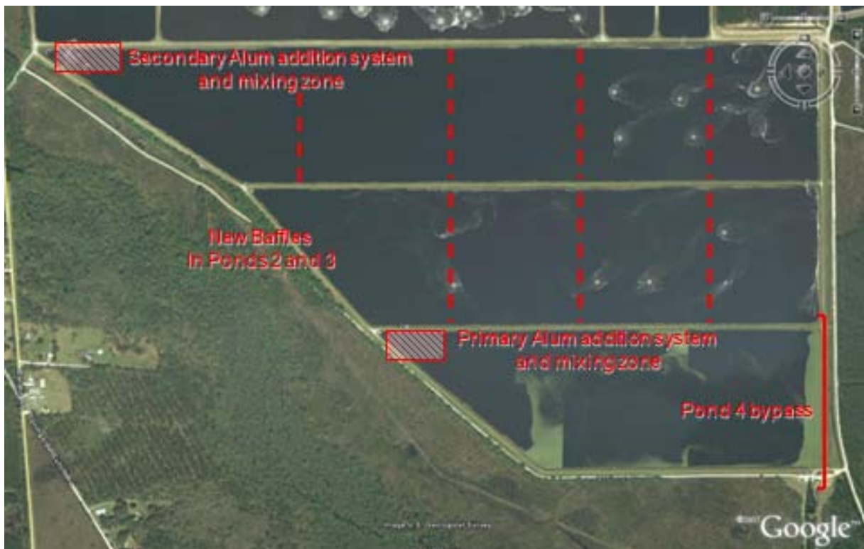
Figure 5-8. Layout of coagulant to Pond 3 effluent
