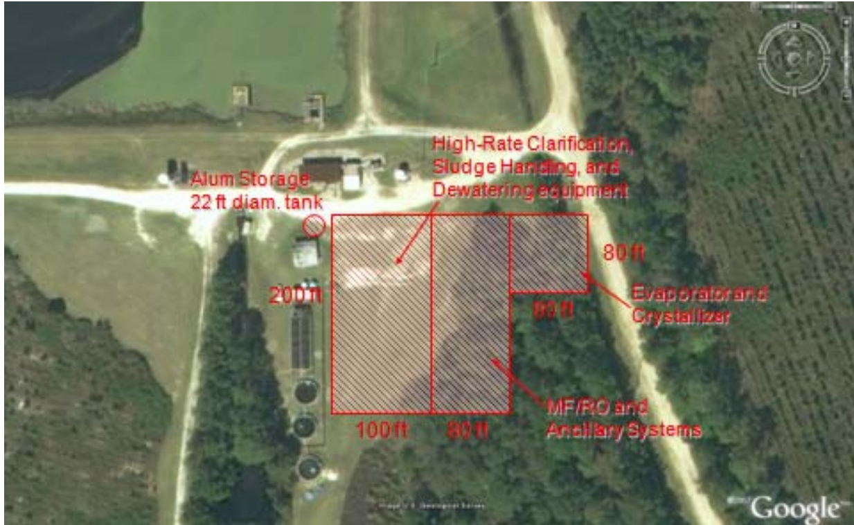
Figure 5-12. Location and footprint of MF, RO, and ZLD system
