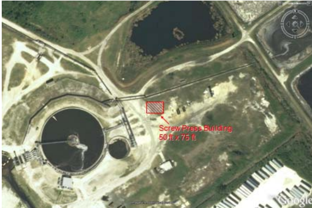
Figure 5-5. Footprint requirements for dewatering primary clarifier underflow
