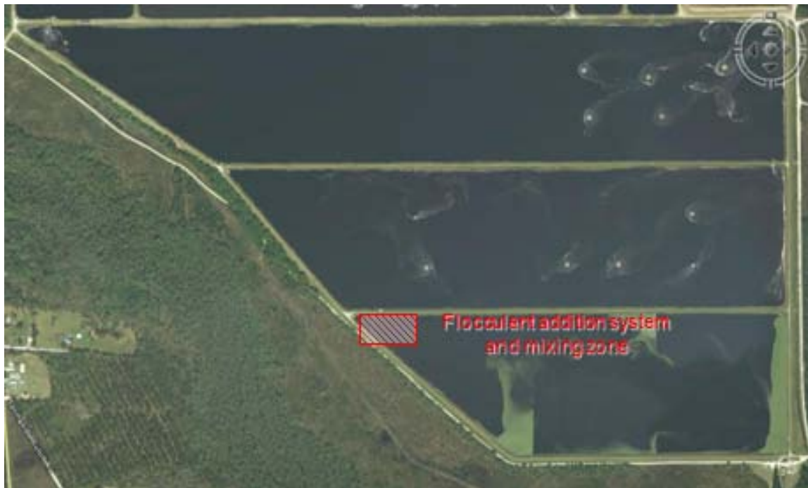
Figure 5-10. Layout of flocculent to Pond 3 effluent during peak TSS events
