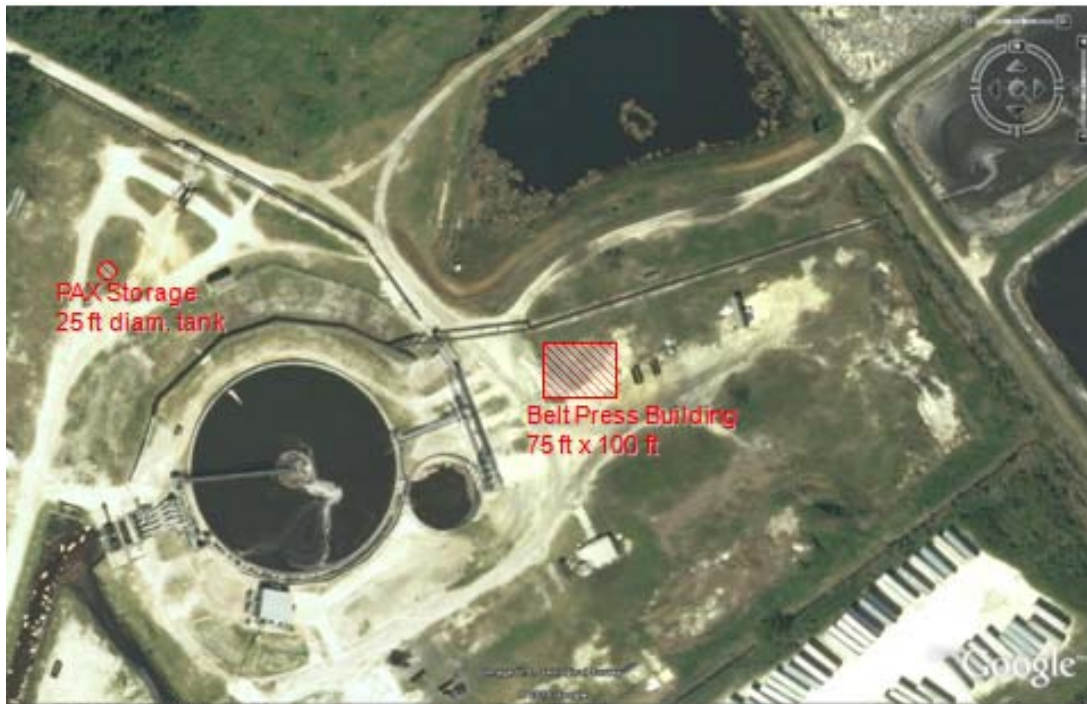
Figure 5-5. Footprint requirements for dewatering primary clarifier underflow
