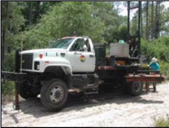
One of the FGS drill rigs used for coring in Manatee Spring State Park.
