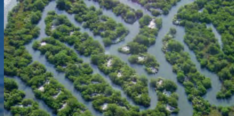
Dragline ditching historically created for mosquito control
