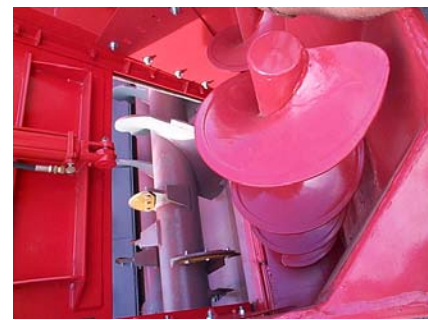
Feed Mixer Auger System. These machines can mix up feedstock and ready it for vermicomposting.
