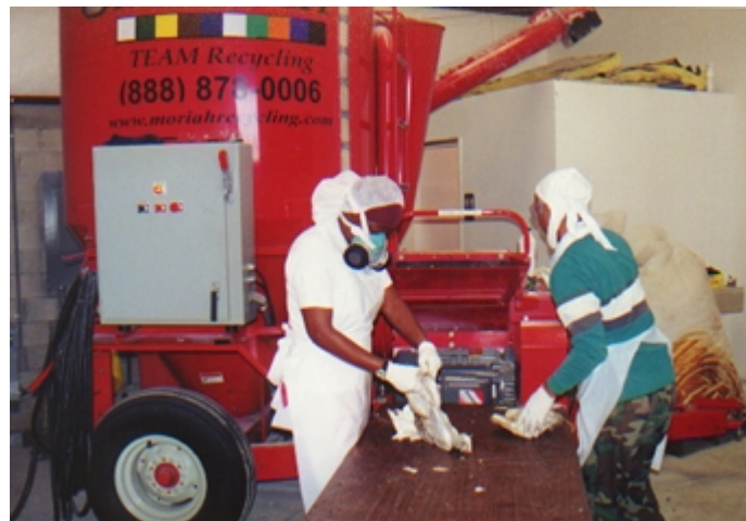
Polystyrene food trays being fed into the grinder.
