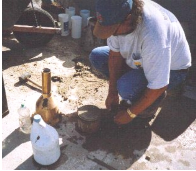
Pouring polystyrene/concrete mixture into the air apparatus.
