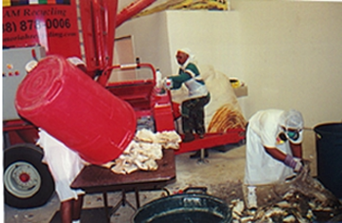
Polystyrene food trays being prepared for grinding.
