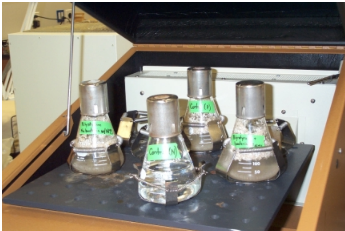
Figure A.1. Flasks prepared with salts, autoclaved polystyrene material and endemic bacterial species from a local lake on the agitator.
