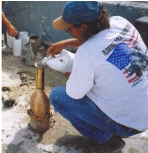
Addition of water to concrete/polystyrene mixture in the air apparatus.
