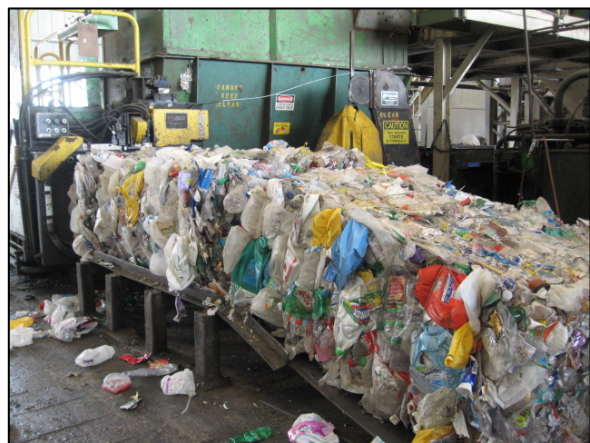
Figure 3.2: Baled HDPE at Orange County MRF
