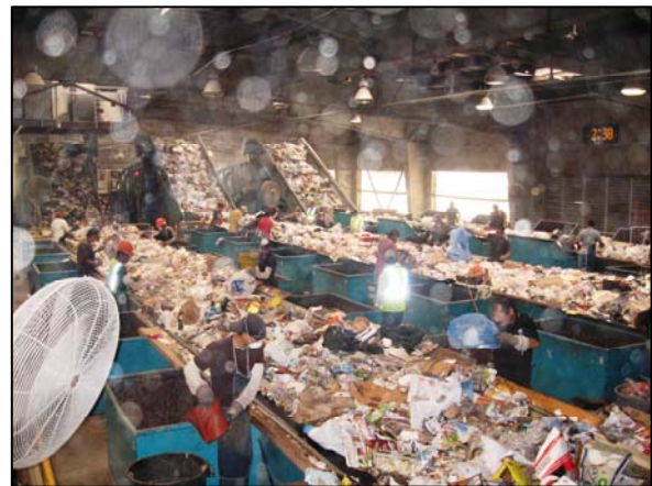
Figure 3.15: Presort Lines at Athens MRF
