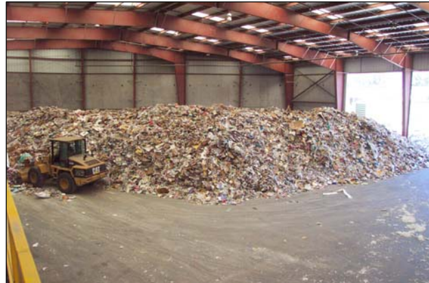
Figure 2.1: Typical Tipping Floor
