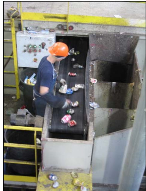
Figure 3.20: Quality Control Following Eddy Current
