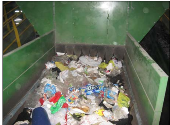
Figure 3.12: Materials Exiting Nihot Drum Separator
