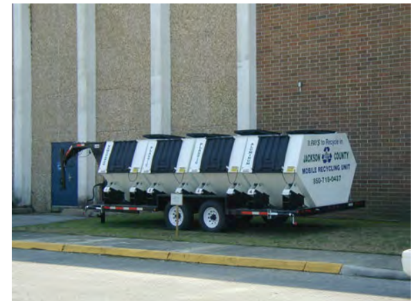
A multiple bin trailer for the collection of Plastic, Aluminum and paper
