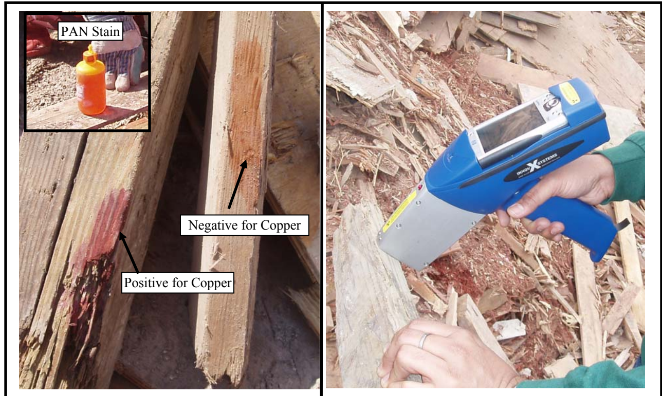
Figure 4: Illustrations of Augmentation Technologies Used in this study. PAN Indicator Stain (left) and hand-held XRF units (right).
