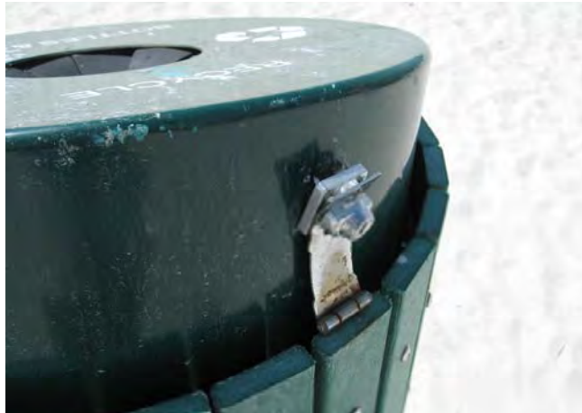
Figure 3.1: Vandalized Lock on Fibrex RPL Container at St. Pete Beach
