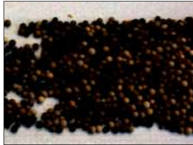
Figure 2.1, 2.2 & 2.3. Heavy tar fouls equipment, left to right: a water scrubber grid, soot formation on catalyst & a gas engine intercooler
