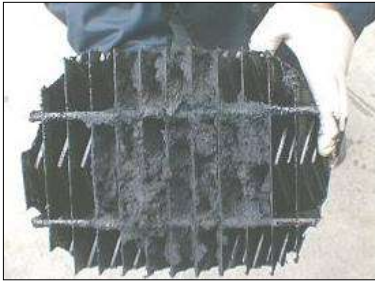
Figure 2.1, 2.2 & 2.3. Heavy tar fouls equipment, left to right: a water scrubber grid, soot formation on catalyst & a gas engine intercooler
