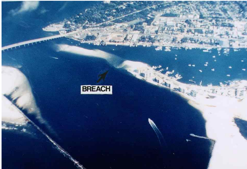
Figure 53. Aerial view of erosional breach through Norriego Point connecting Destin-East Pass with Old Pass Lagoon (closed by USACOE after storm).
